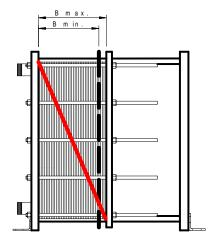
5. Take the tensioning screws out of the loose plate.
